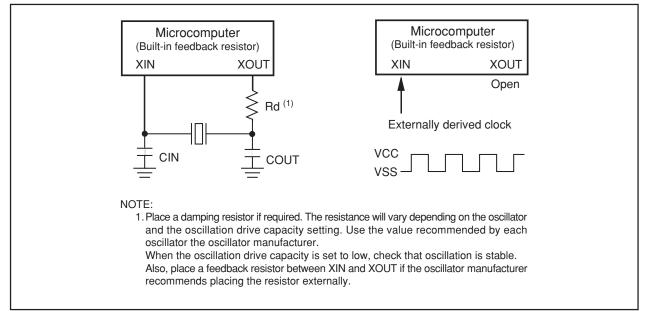
Figure 7.9 Examples of Main Clock Connection Circuit
